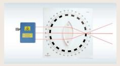
Equipped with a key switch and a AC adapter 220V / 3 V DC.
